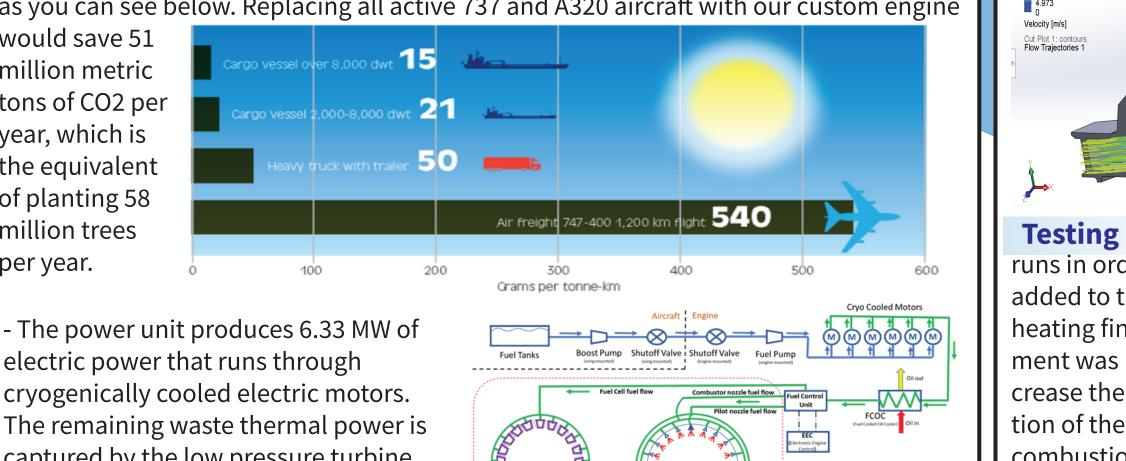
electric power that runs through cryogenically cooled electric motors. The remaining waste thermal power is captured by the low pressure turbine and transferred to the low pressure shaft. You can see our Hydrogen Fuel System to the right.
